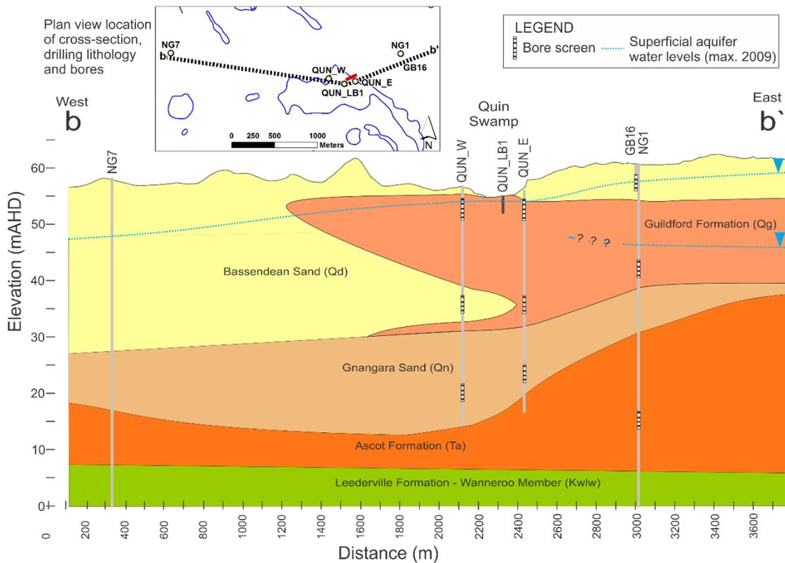
Figure 13 Interpreted local geology and hydrogeology cross-section including monitoring bores for Quin Swamp
