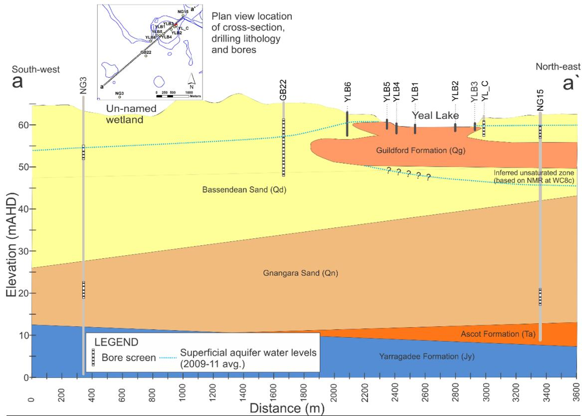
Figure 11 Interpreted local geology and hydrogeology cross-section including monitoring bores for Yeal Lake
