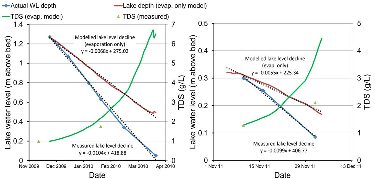
Figure 17 Measured and modelled evaporation only decline in water levels following cessation of surface inflow to Yeal Lake in 2009 and 2011
