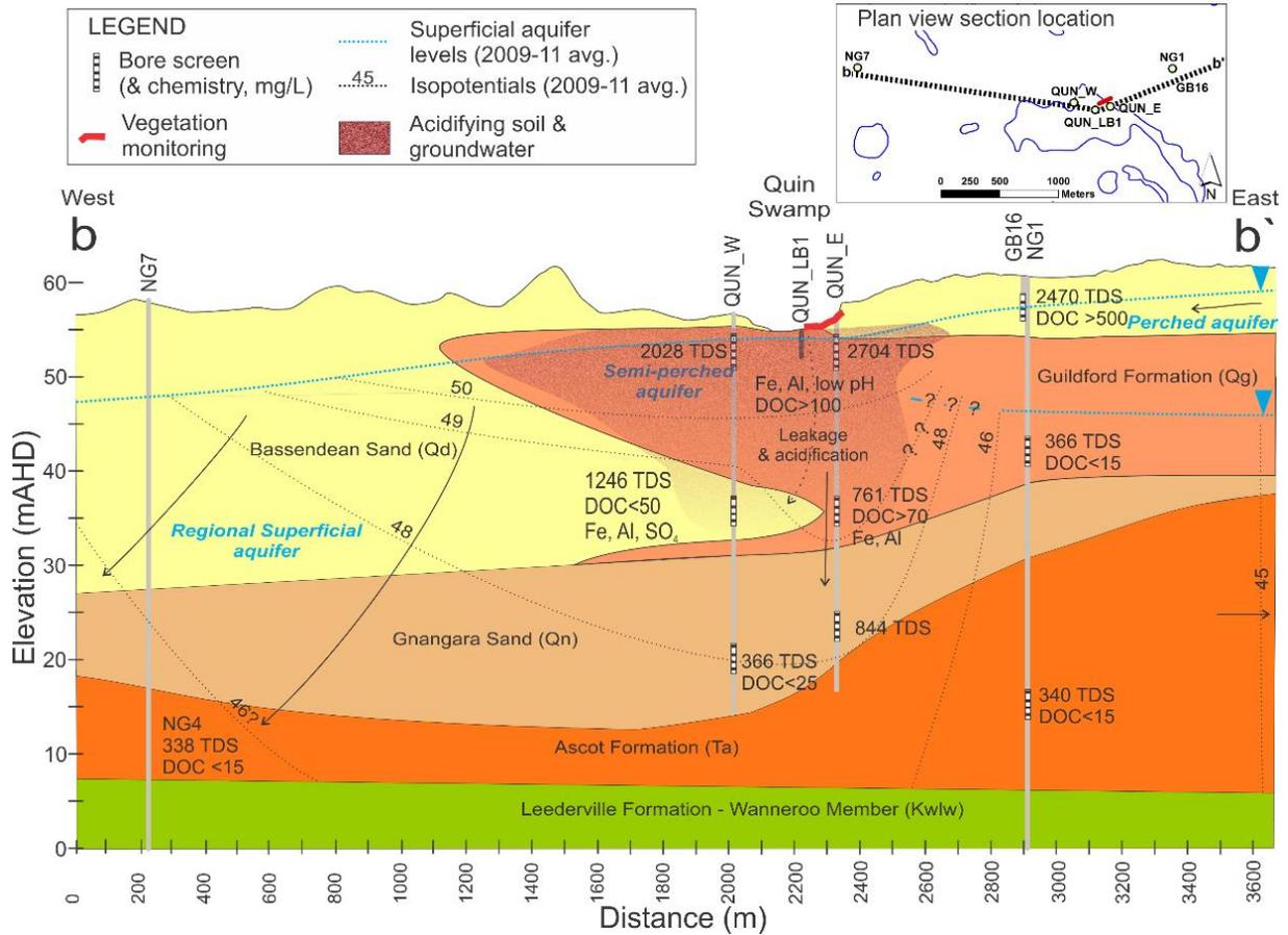
Figure 26 Cross-section of the local hydrogeology of Quin Swamp with interpreted groundwater flow paths
