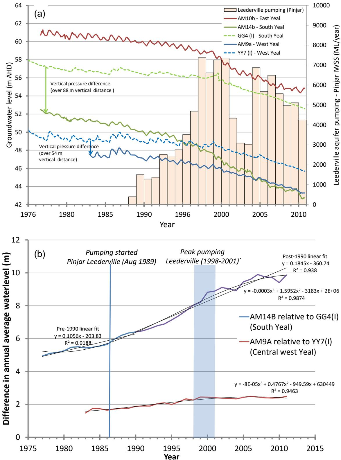
Figure F1 Leederville aquifer and corresponding deep Superficial aquifer water levels (a) and average annual pressure difference (b) in relation to pumping at the IWSS Pinjar borefield (> 6 km south).
