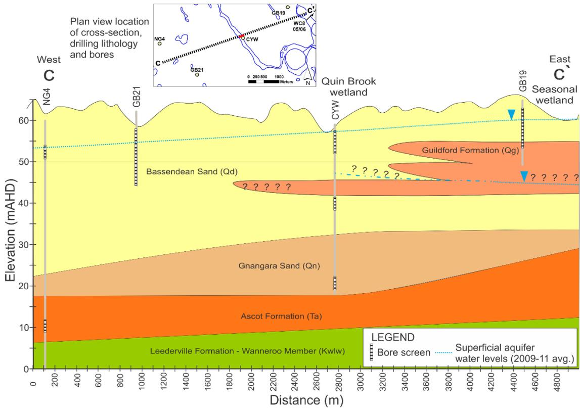
Figure 12 Interpreted local geology and hydrogeology cross-section including monitoring bores for the upper Quin Brook wetland
