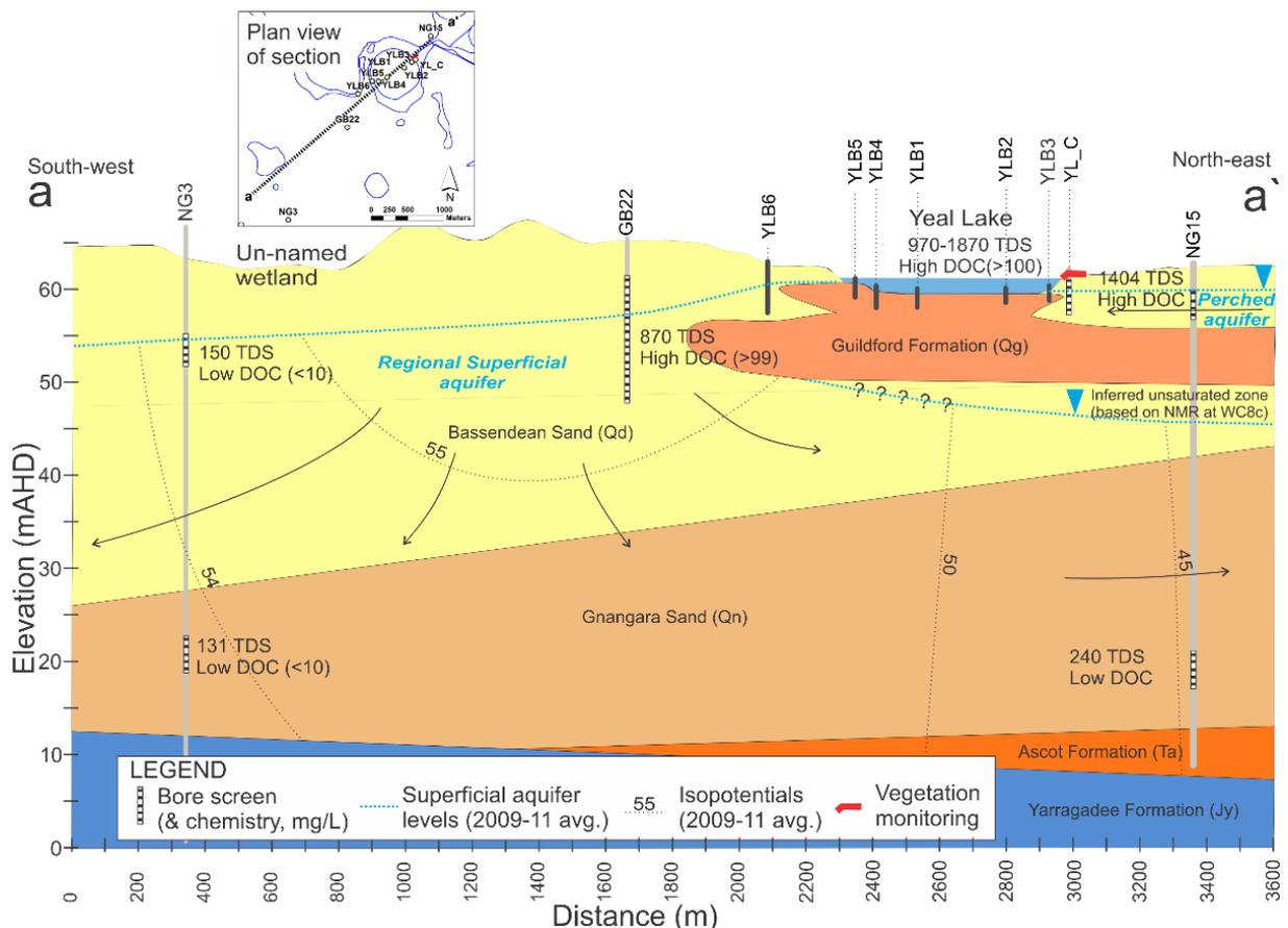
Figure 24 Cross-section of the local hydrogeology of Yeal Lake with interpreted groundwater flow paths
