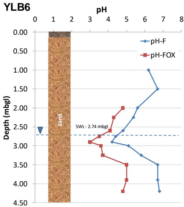
Figure D1 Field (F) and peroxide (FOX) oxidised pH, summary lithology, potential (Scr) and available (TAA) acidity analyses (moles H<sup>+</sup>/tonne) in Yeal Lake. Note: no ANC in any samples.
