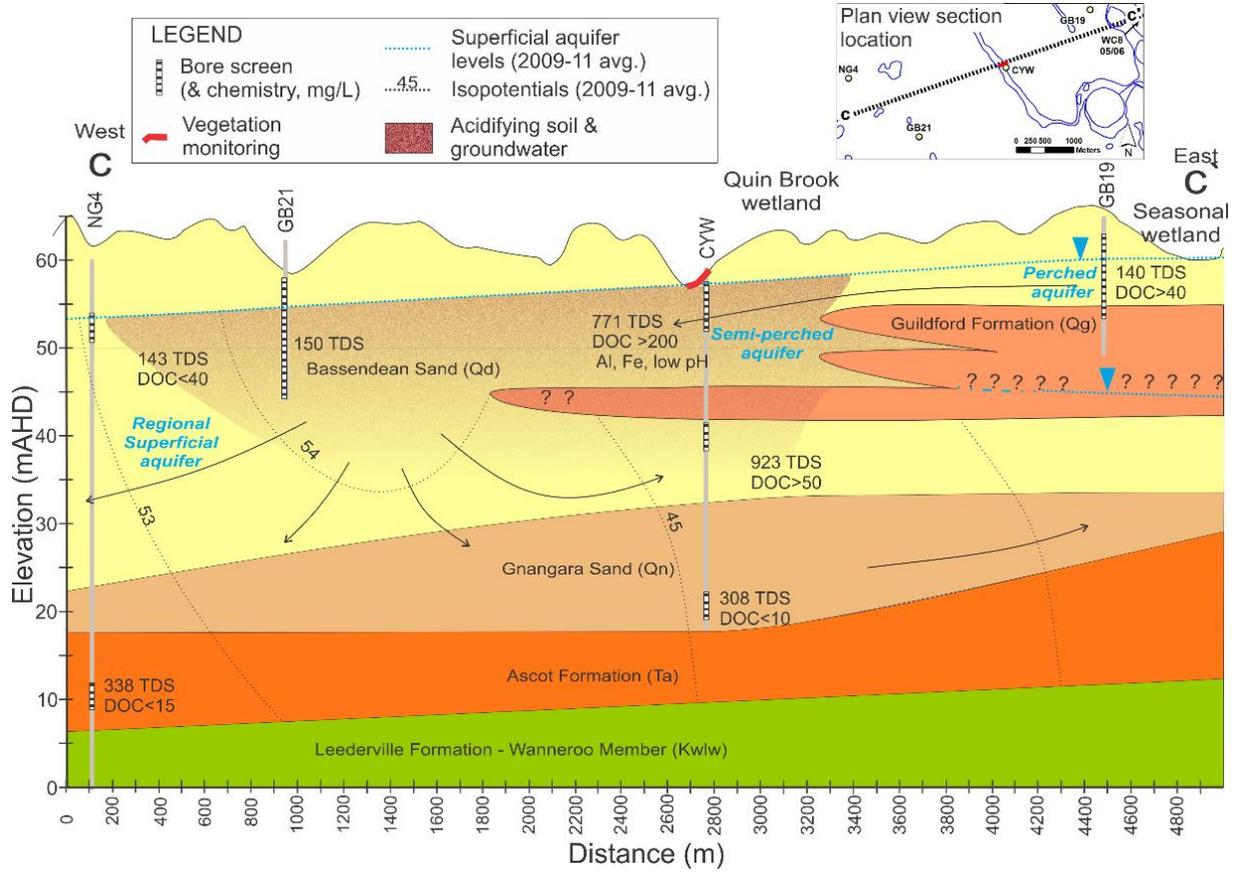
Figure 25 Cross-section of the local hydrogeology of upper Quin Brook wetland with interpreted groundwater flow paths
