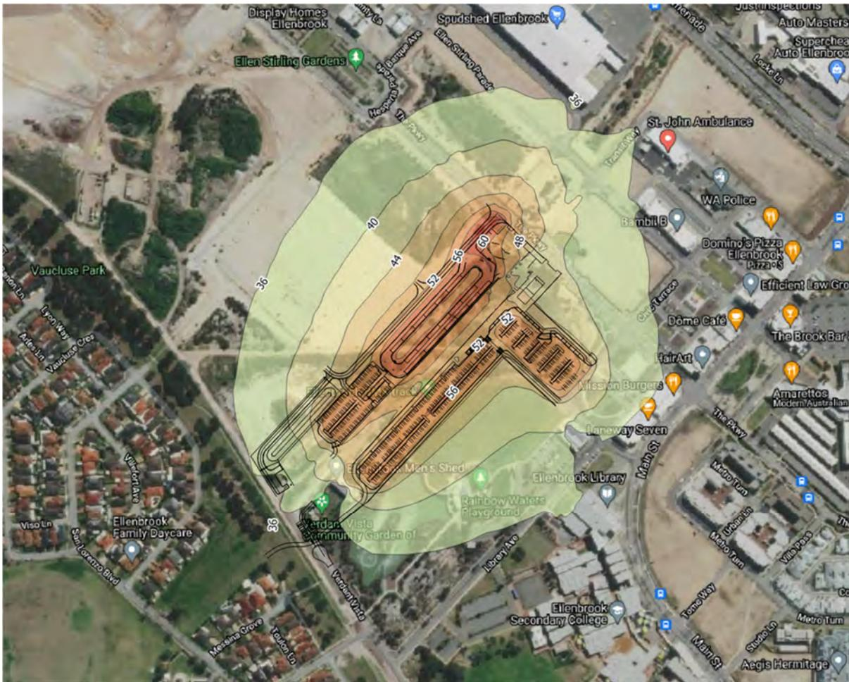
Figure 8: Indicative distribution in airborne noise from station, bus and car parking areas for comparison with  $L_{Aeq}$  criteria
