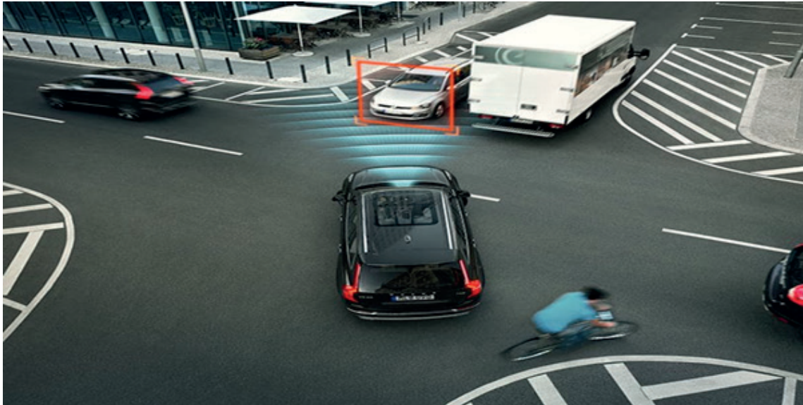
Fig 3: Intersection Collision Warning System
