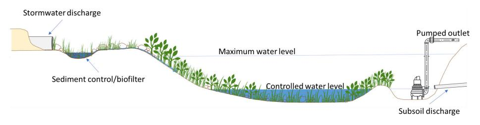
Figure 31: Schematic representation of detention storage and discharge pump system at a local hub
