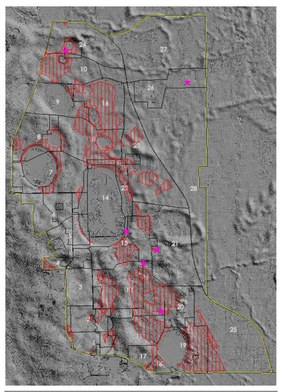
Figure 30: Development areas at risk from rising groundwater levels where subsoil drains should be installed and later utilised to harvest water for reuse (pink stars indicate potential contamination sources (DWER, 1991)
