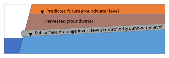
Figure 29: Schematic representation of estimated harvested groundwater
