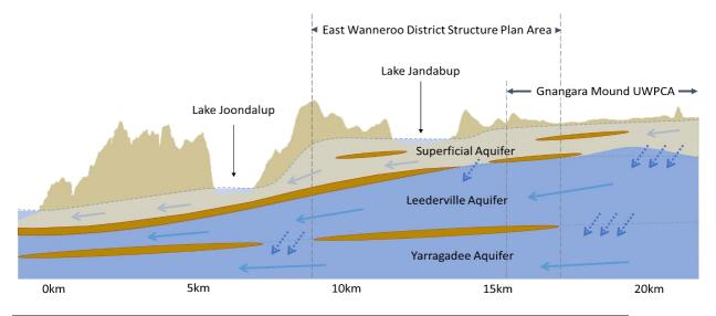
Figure 10: Schematic cross section through the site and underlying groundwater system
