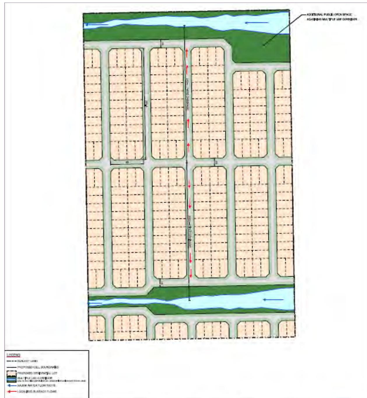
Figure 2.12: Typical residential lot and swale layout for Wanju (IWMS, 2015)
