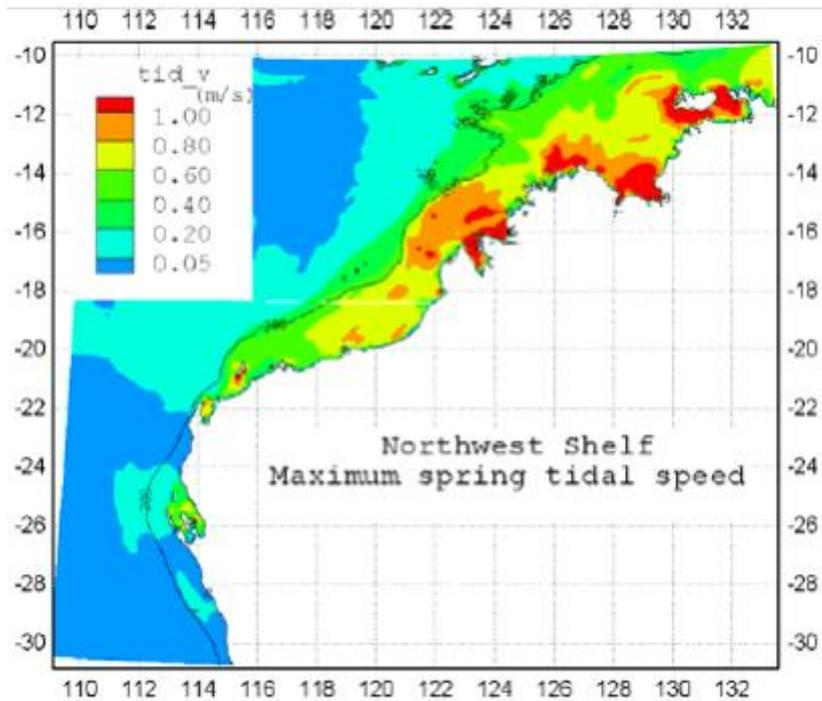
Figure 4-10: Depth-Averaged Maximum Spring Tidal Speed (Li *et al.* 2008)
