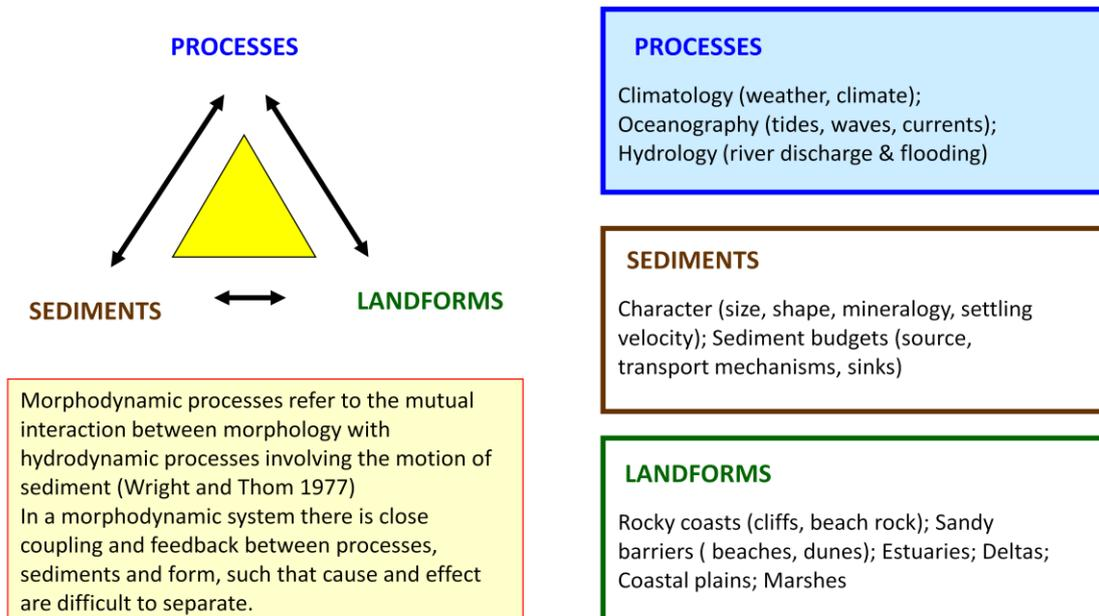
**Figure 2-5: Components of a Morphodynamic System on a Sandy Coast**
