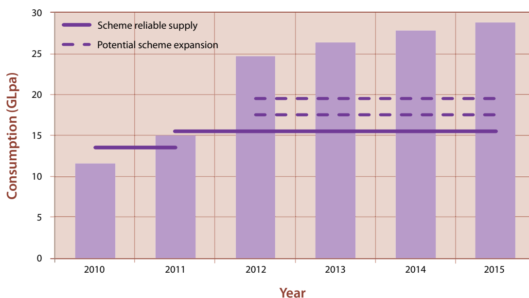
Figure 4.2. Port Hedland Water Supply Scheme: water requirements to meet demand (2010-2015)
