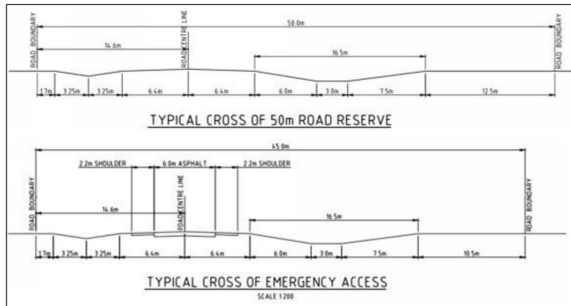
Figure 15 - Indication of typical internal road geometry compiled from eastern GIA Engineering Report (Cossill & Webley, 2013)
