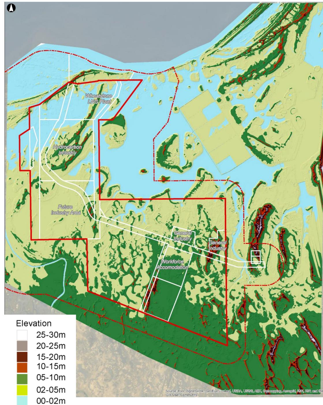
Figure 4 – GIS output showing Lidar elevations indicating low lying and natural high ground in relation to future areas of development at the ANSIA.
