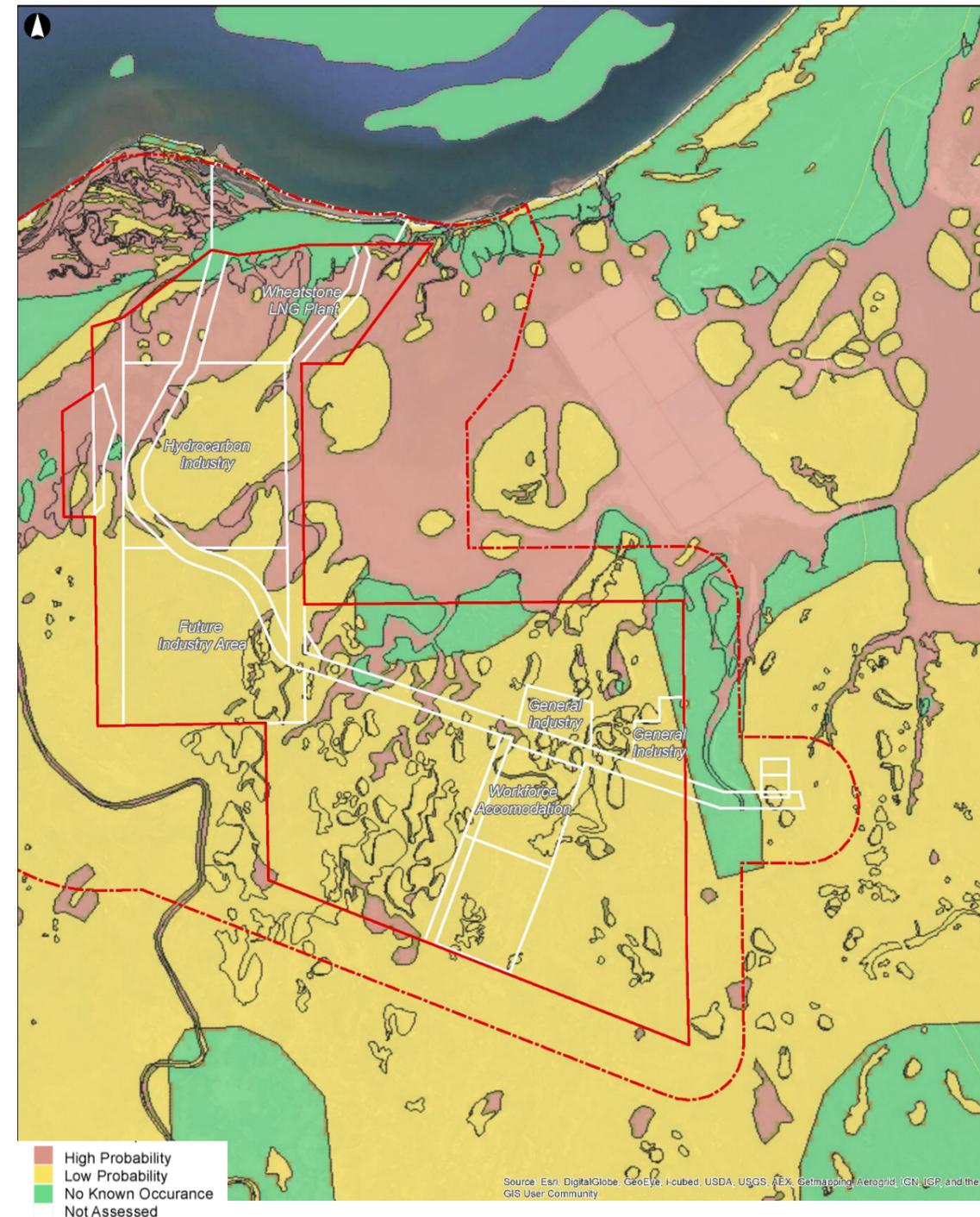
Figure 10 – GIS output showing Acid Sulfate Soil risk areas (Australian Soil Resource Information System, 2014) in relation to future areas of development at the ANSIA.
