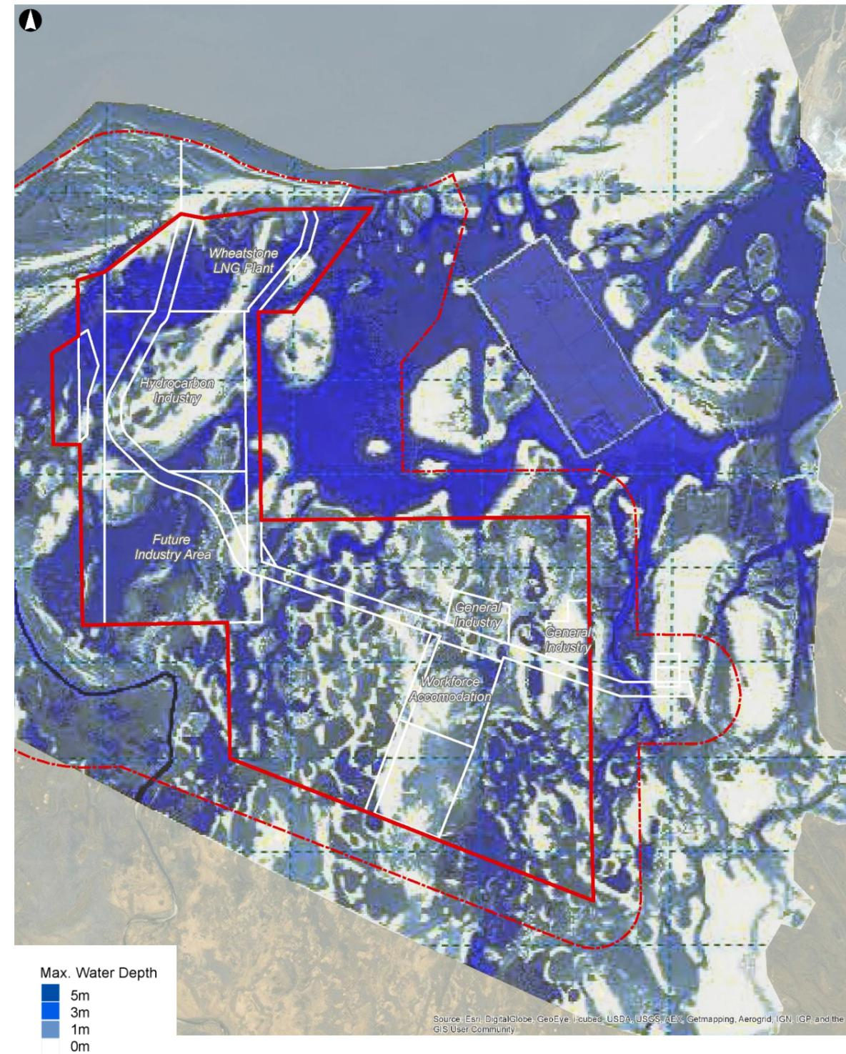
Figure 7 – GIS output showing Surface Water Studies pre-development scenario max. water depths (100year ARI) relative to future stages of the ANSIA (URS, 2010a)
