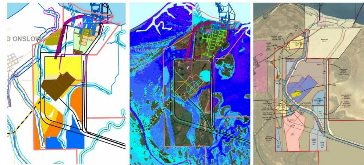
Figure 6 Series of report images showing how natural channels identified within the hydrological study (left and middle) (BG&E, 2011c) shaped part of the Stage 1B & 1C Development Plan (right) (TPG, 2012)
