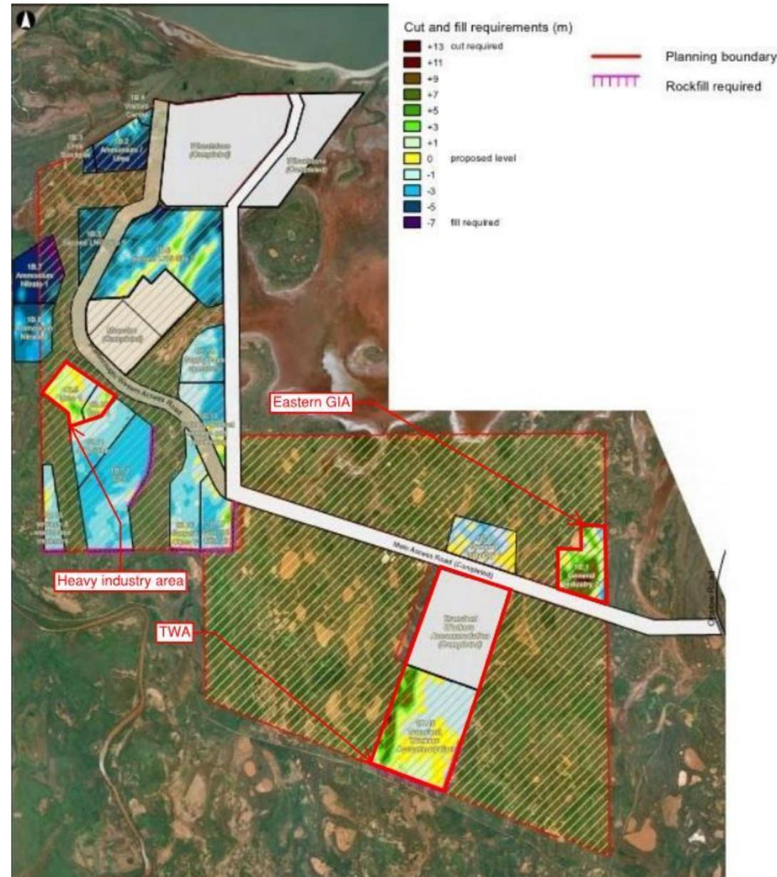
Figure 12 – Annotated extract of Fill Sourcing Study indicating cut-fill requirements from previous stages of the ANSIA , where green and brown indicates cut, blue indicates fill, and yellow is already balanced (Arup, 2014).
