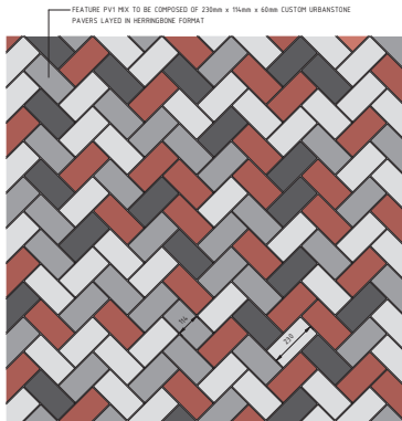
1 YRE PAVING DETAIL 1 - PV1 FEATURE MIX SCALE 1:10
