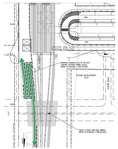
Figure 44. Yanchep Station – PSP Alignment and Ramp Arrangement
