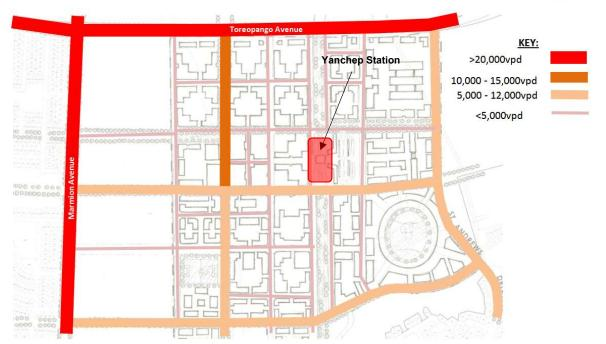
Figure 12. Yanchep Activity Centre Structure Plan – Forecast Traffic Projections
