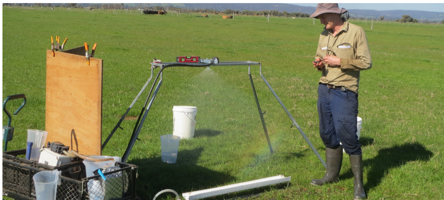
A department scientist uses a rainfall simulator to measure phosphorus loss from saturated soil.
