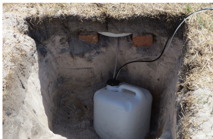
A catchpan and drum (lysimeter) installed to collect water that has leached through the top soil.
