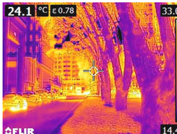
Figure 3. Thermal image of shaded Victoria Avenue in the City of Perth. Ambient air temperature is 31° Celsius. Temperatures range from 14.4° C in the shade to 33° C in unshaded areas. The temperature in shaded areas was an average 6° C cooler. 9
