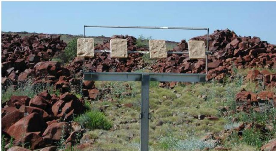
Figure 2 Exposure rack with collector tiles at Dolphin Island (Source: CSIRO 2007a)
