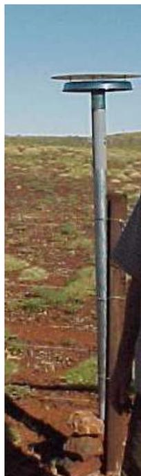
Figure 3 *Passive samplers under lid with aluminium radiation screen (Source: CSIRO 2010a)*
