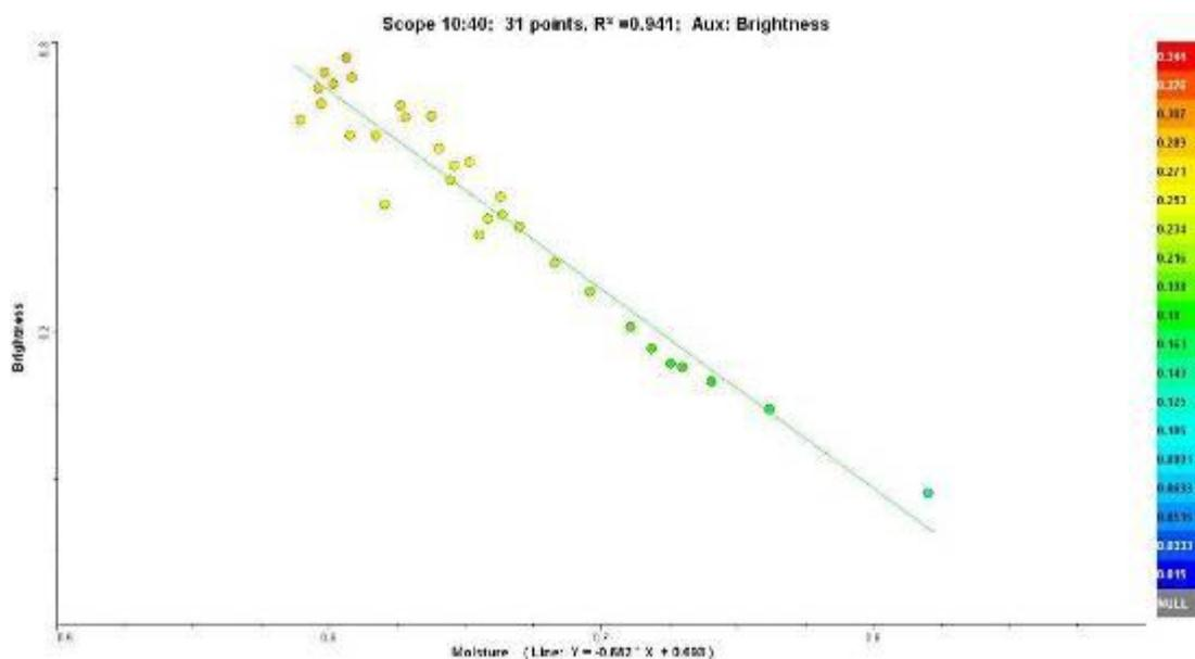
Figure 12. Scatterplot of brightness versus moisture (depth at 1900 nm).
