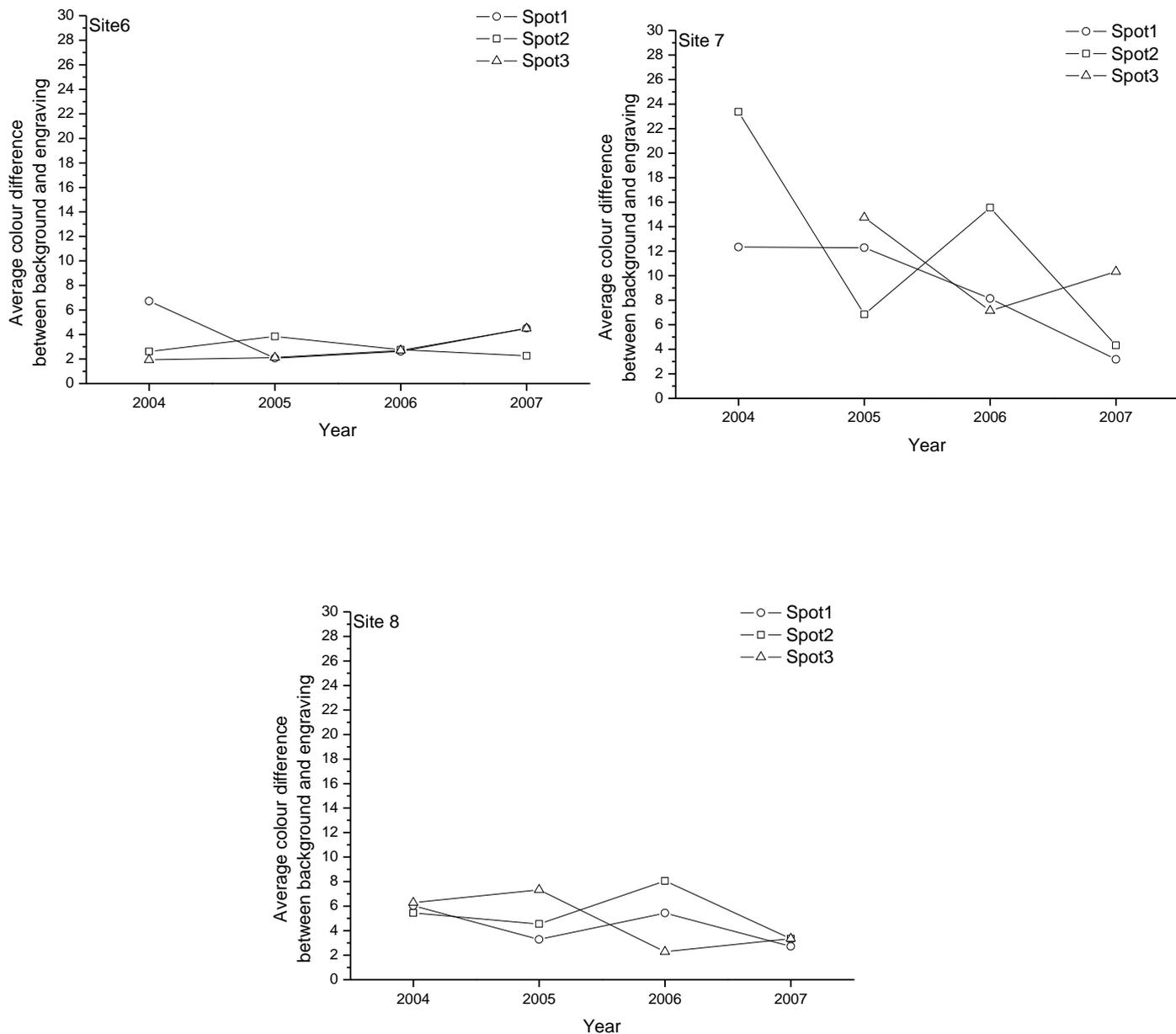
Figure 8: Site specific plots of colour differences between engraving and background for each spot examined (2004–2007). Site 5 spot 3 and Site 7 spot 2 are believed to exhibit high variance due to measurement effects.
