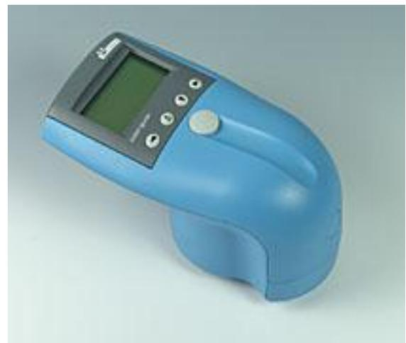
Figure 1: Portable spectrophotometer used for colour measurements.
