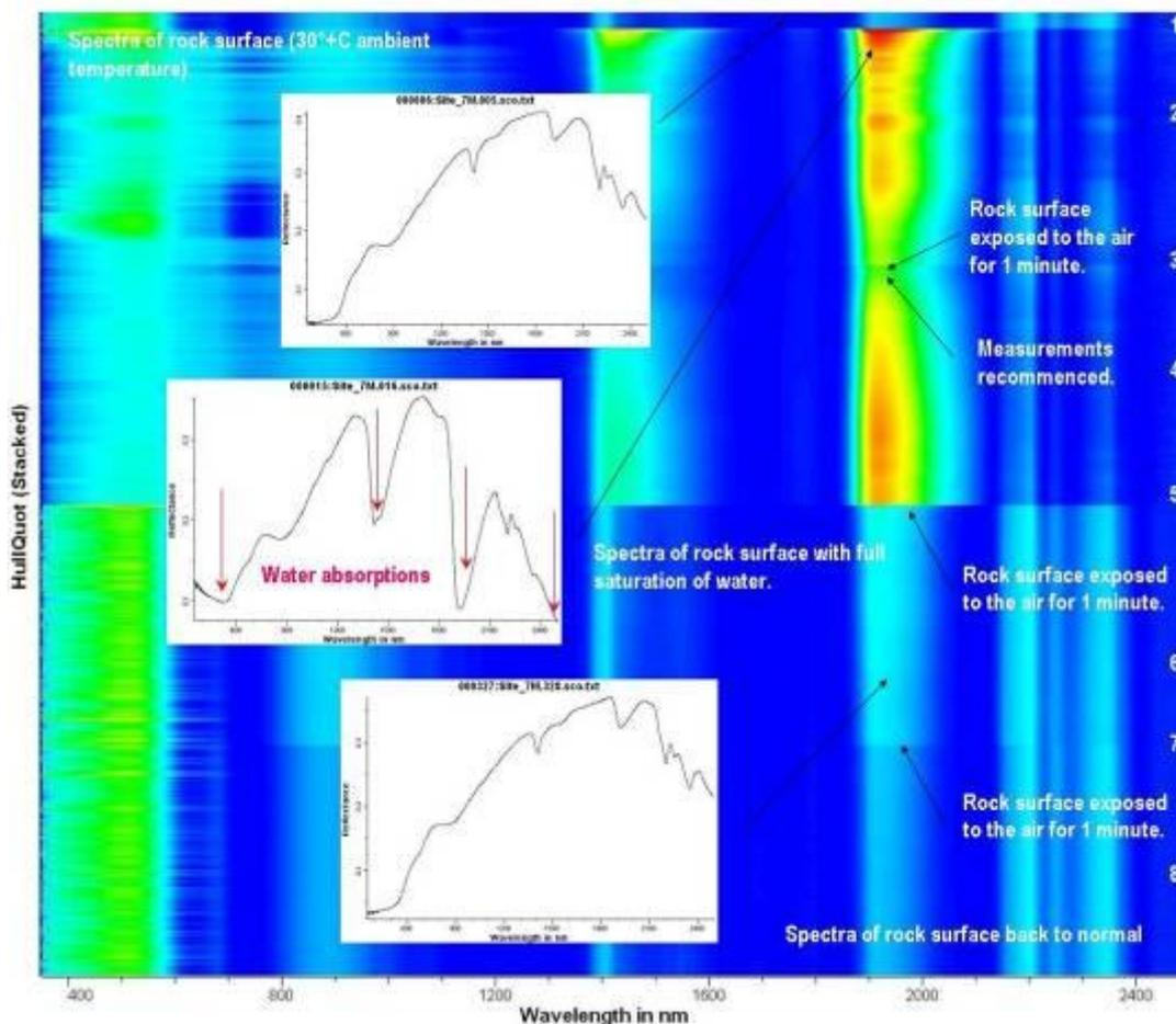
Figure 11. Image plot and spectra for the water experiment.
