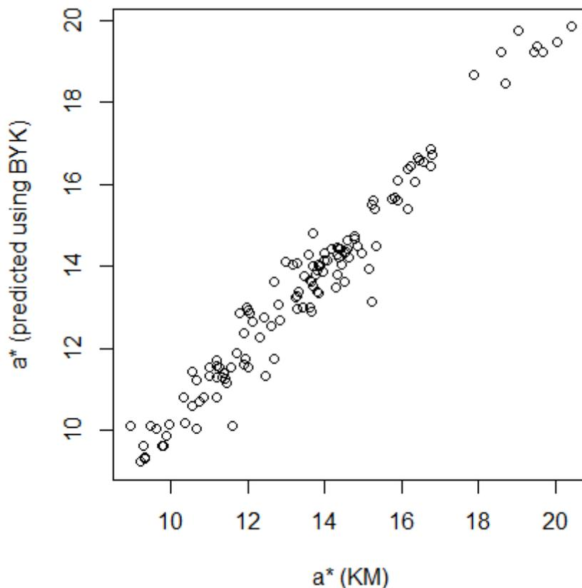
**Figure 33: a\* measurements on the KM machine and their predictions using BYK observations**
