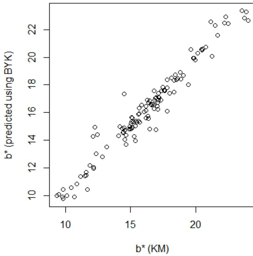
Figure 34:  $b^*$  measurements on the KM machine and their predictions using BYK observations.
