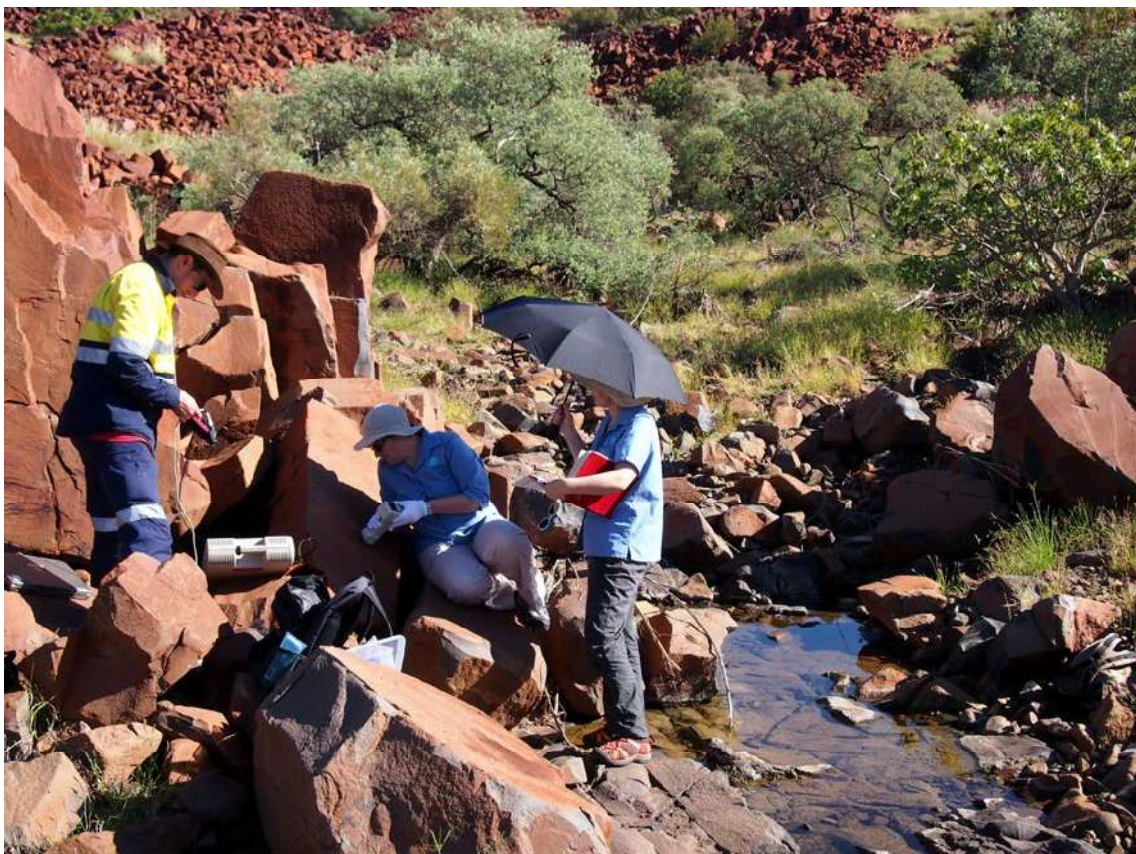
Figure 27: ASD FieldSpecPro and Konica Minolta CM-700dspectrophotometer operating on petroglyphs in the Burrup Peninsula (2013)
