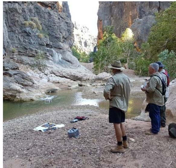
This hydraulic model required a high resolution digital elevation model (HRDEM) to define the geometry of the gorge. In developing the model, we used a drone and image recognition technology to capture a point cloud (a set of data points in space) of more than 83 million ground points. We used GIS software to post-process the point cloud to produce an HRDEM suitable for our purposes.
