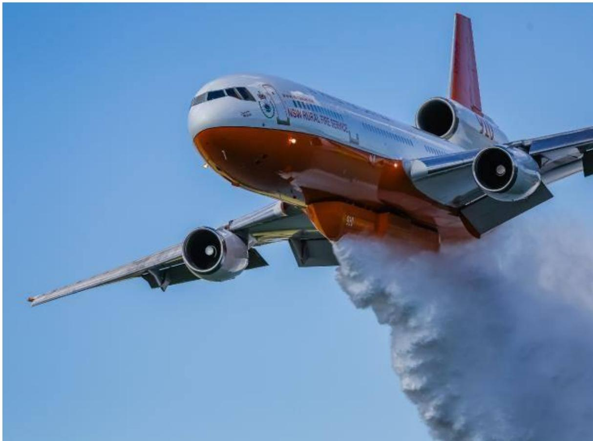
The DC-10 air tanker was developed by 10 Tanker Air Carrier LLC, an American company. Over a period of 10 years, 10 Tanker developed the DC-10-10 and later the DC – 10-30.
