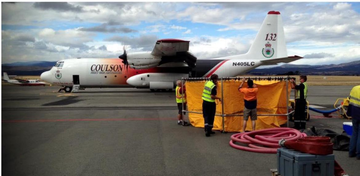
The example above showed the setting up of portable equipment for the LL-100 Hercules deployed to Tasmania in February 2016. The Hercules was fully filled and operational 32 minutes after arriving in Tasmania, and went on to make a significant difference to these fires using equipment carried on board or procured from local hire companies.
