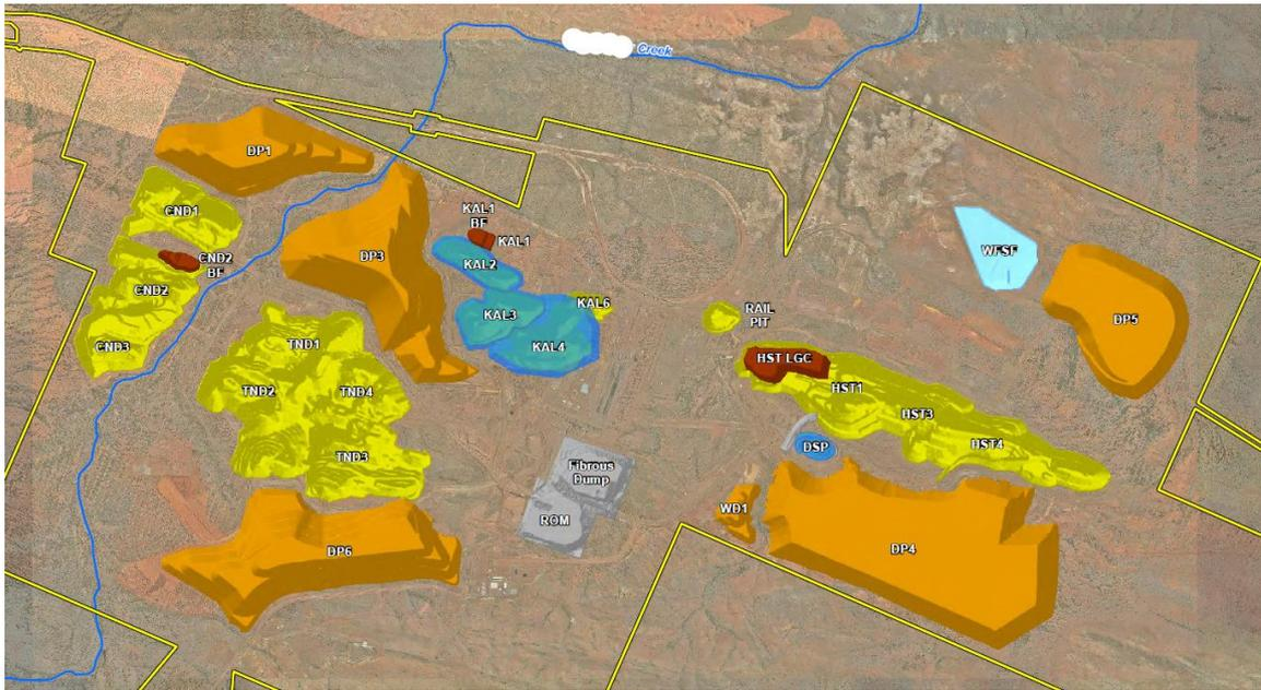
Figure 4. Example of rehabilitation and design diagrams for mining landforms to remain post closure.
