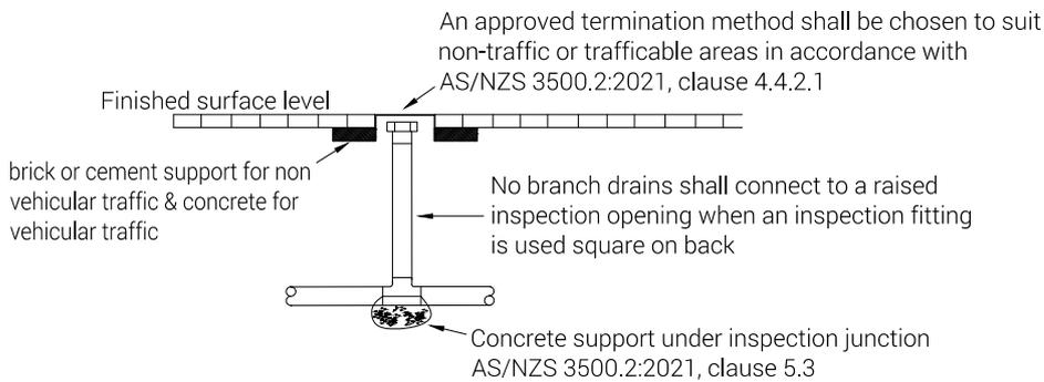
**Diagram 2:** Typical raised inspection opening
