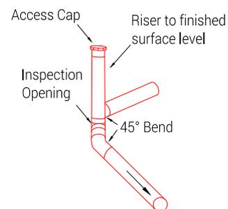
**Diagram 6:** Preferred method of providing raised access into drain
