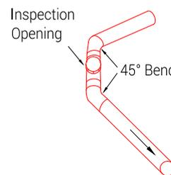
**Diagram 5:** Preferred method of providing access into drain
