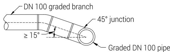
**Diagram 8:** Connection of DN 100 pipes with a 45° junction inclined at 15° where WC pans are connected upstream
