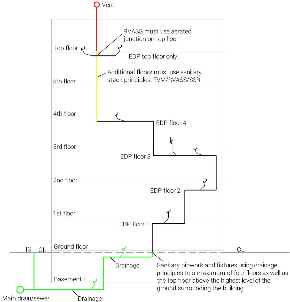
**Diagram 6:** Shows the point at which EDP commences when buildings have floors below the ground level
