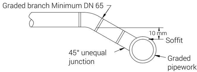
**Diagram 7:** Connection of a branches using an unequal 45° junctions
