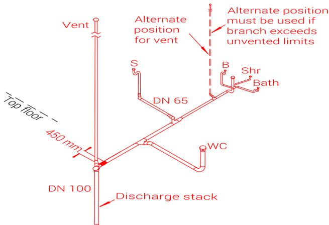
**Diagram 2:** Vent off the discharge stack or upstream end of the branch
