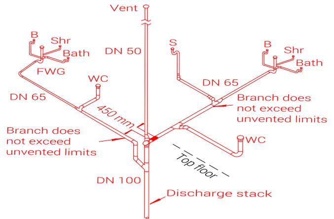
**Diagram 3:** Vent off the discharge stack with branches under unvented limits
