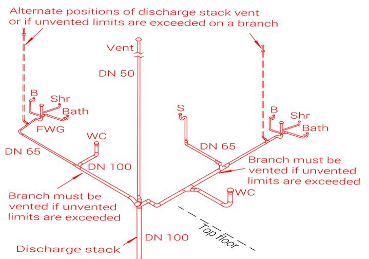
**Diagram 5:** Vent on the upstream end of either branch where a double junction is used
