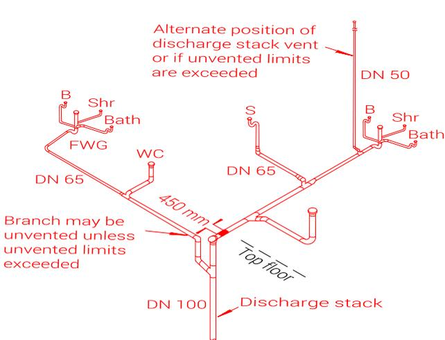
**Diagram 4:** Alternate position of vent on the upstream end of uppermost branch
