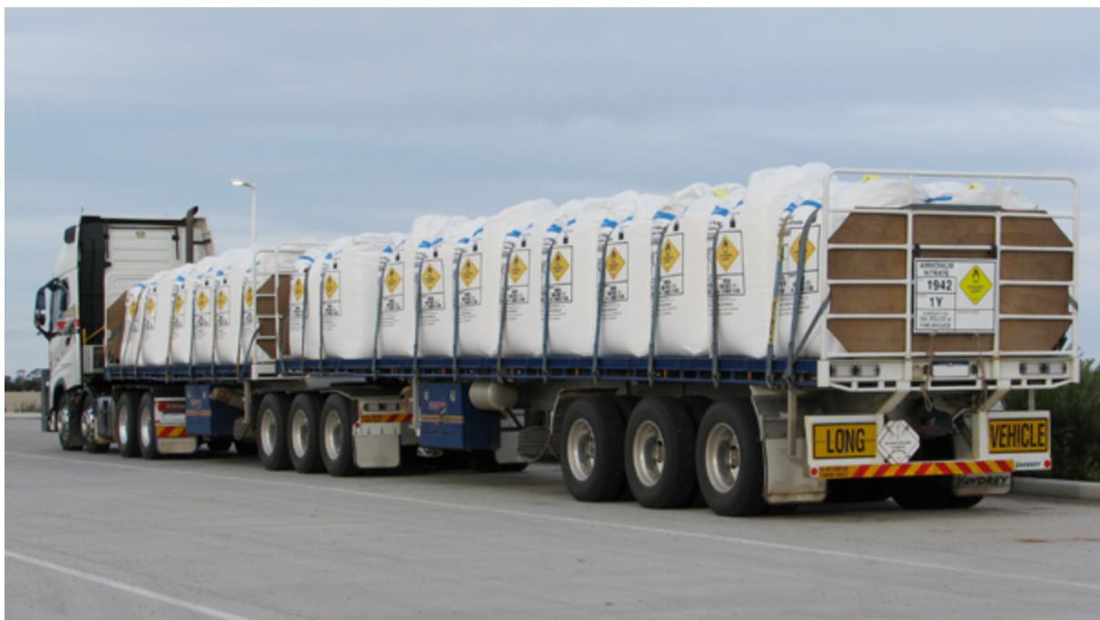
Figure 8.1 AN in IBCs on a combination vehicle
