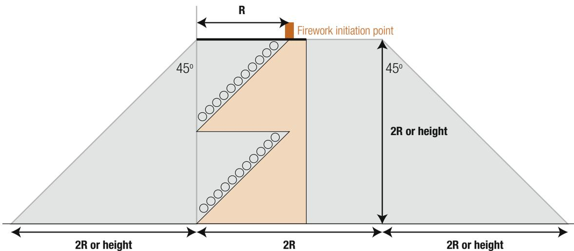
Figure 5.4 Side view showing exclusion zone for ground fireworks on a stadium
